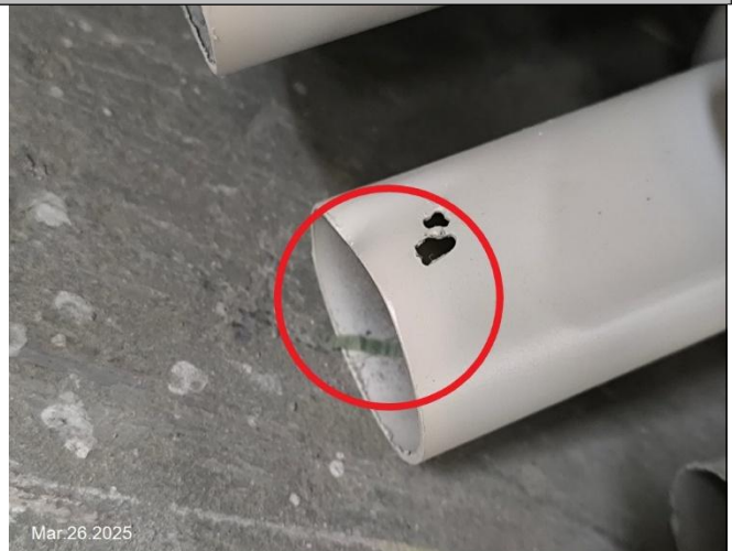
Major Defect-Deformed on end of pole
