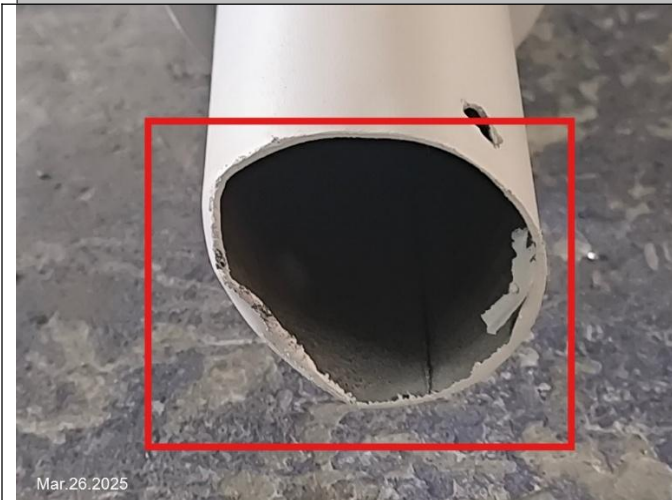
Major Defect-Deformed on end of pole
