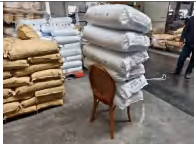
Load Capacity Test
