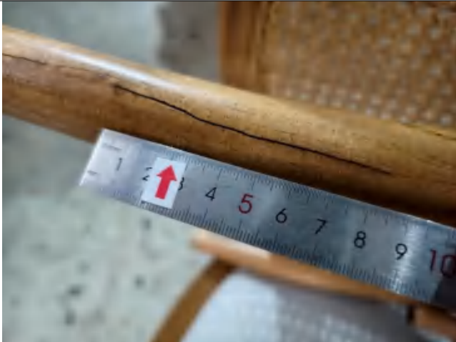
Crack on surface-Maj
